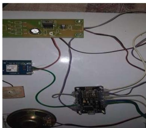
Fig. 7. Node MCU with GPS Module
